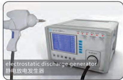
electrostatic discharge generator
